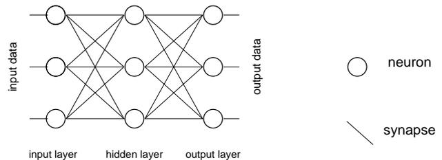
Fig.1: Multilayer perceptron, which is a nonlinear network that consists of an input layer, an output layer, and one hidden layer. One hidden layer is sufficient in order to be a universal approximator for any continuous nonlinear function.
