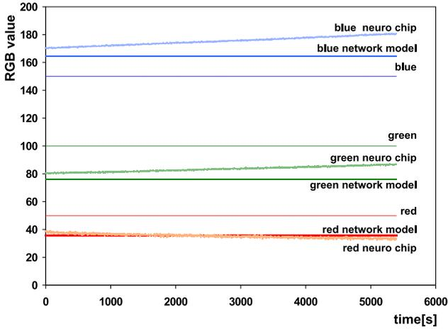
Fig.4: The color curves over a period of time of over 1.5h for the network model (software) and the neural network chip; the drift appears by unloading of the storage capacitors of the chip.
