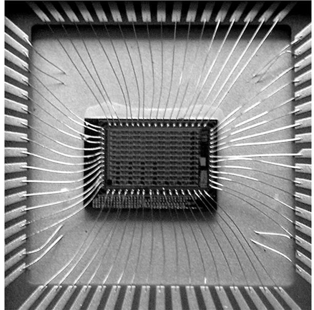
Fig.5: Analog Neural Network Chip with the topology of 10 input neurons, 6 hidden neurons and 10 output neuron. The number of synapses amounts to 136. The size of the die is approx. 10 mm<sup>2</sup>.
