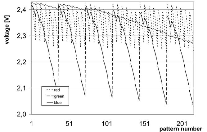
Fig.3: Sensor voltages of TFT-monitor measurement for RGB values between 0 and 250 in steps of 50.
