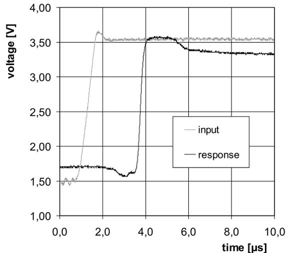
Fig.6: Measuring results shows a pin to pin response time of approx. 5  $\mu$ s. The output currents of  $\pm 500 \mu$ A are transferred by a transimpedance converter to an output range of 1.5 ... 3.5 V.
