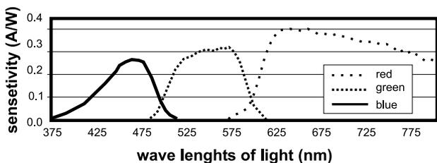
Fig.2: Spectral sensitivity of the sensor outputs [5].
