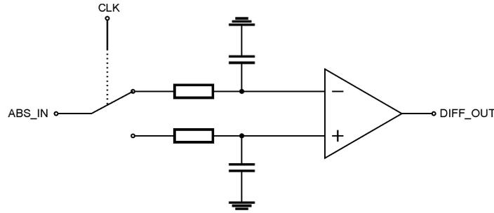
**Fig. 2: Ambient light suppression circuit concept**
