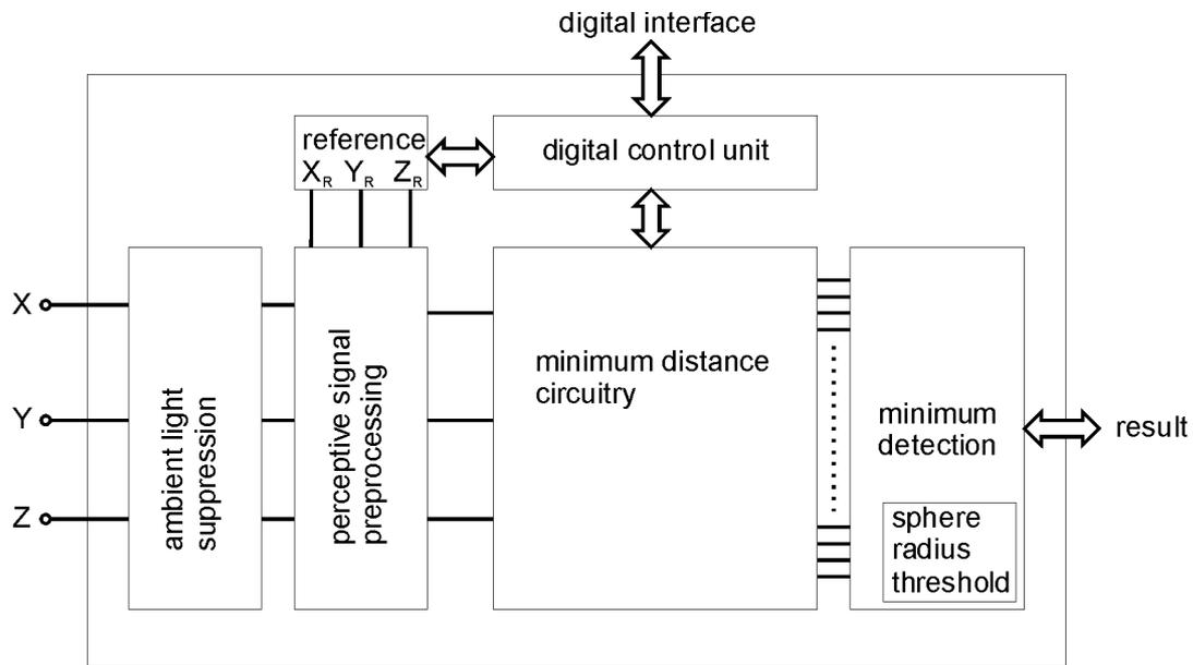
**Fig. 3: Block diagram of the color processor**
