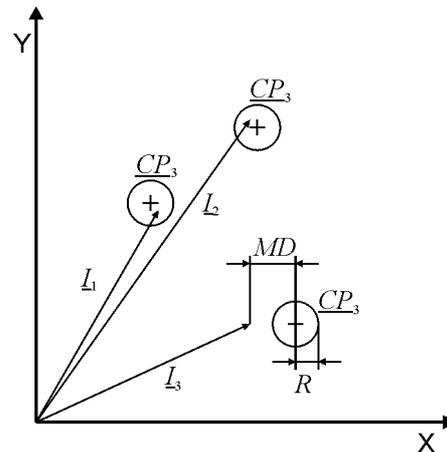
**Fig. 5: Distance diagram for three color patterns and color input vectors**
