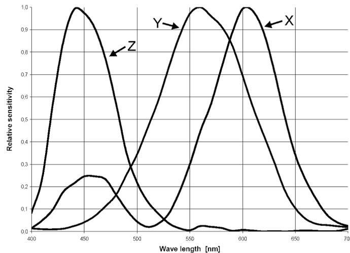
Fig. 1: Normalized filter curves of the true color sensor [2]
