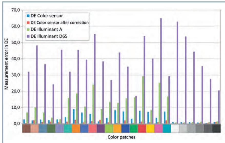
4 Measuring error of color sensor before and after correction, and color variations for illuminants A and D65
