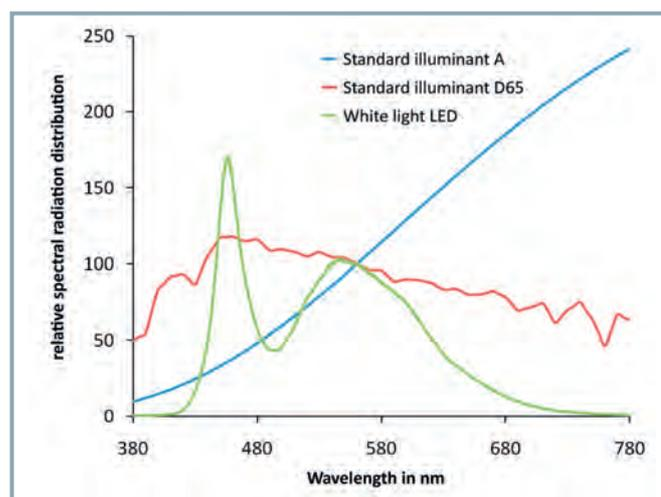
**1** Measured spectrum of a white light LED compared to the standard illuminants A and D65
