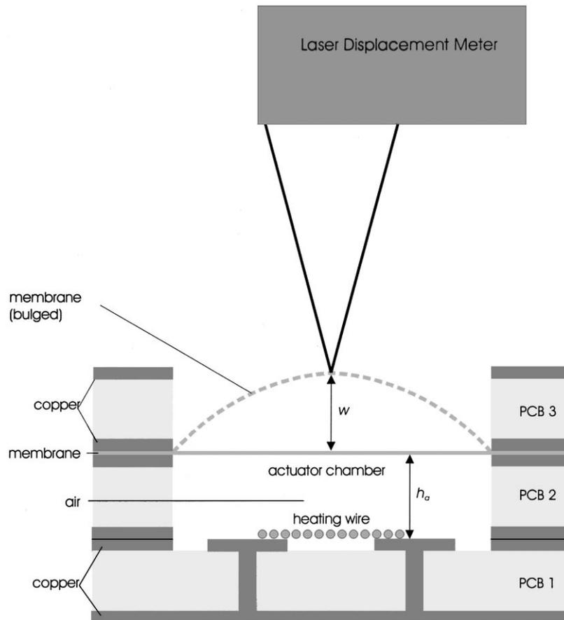
Fig. 3. Schematically cross-section of a thermopneumatically driven volume actuator.
