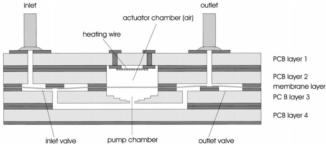
Fig. 1. Schematically cross-section of the micropump.
