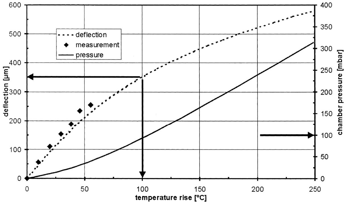
Fig. 4. Theoretical relations of deflection, chamber temperature and pressure of a 10 mm diameter volume actuator and measured deflections at thermal equilibrium.
