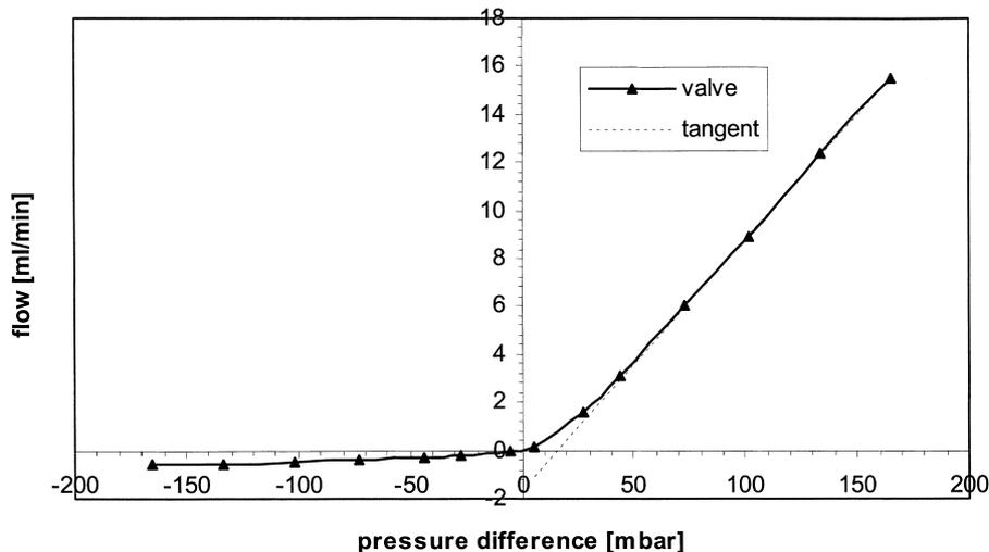
Fig. 7. Characteristic curve of the passive membrane check valve.
