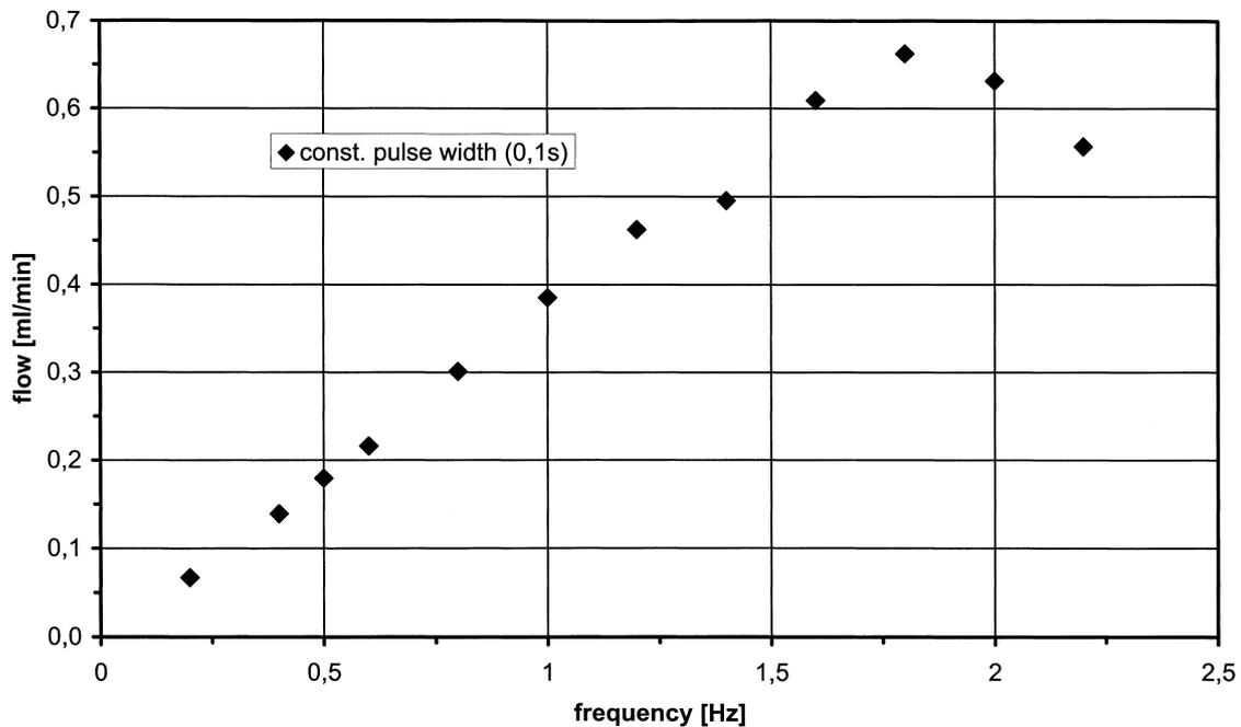
Fig. 10. Flow vs. exciting frequency for constant pulse width (0.1 s).
