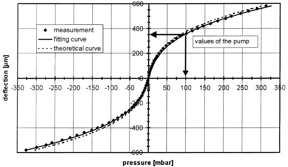
Fig. 2. Deflection curve of a 10 mm diameter Kapton<sup>®</sup> membrane (thickness 7.8 µm).
