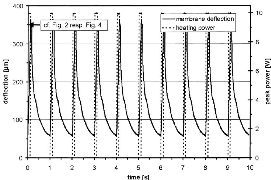
Fig. 5. Dynamically measured membrane deflection of a 10 mm diameter actuator (frequency 1 Hz, duty cycle 0.1, mean power consumption 1 W).
