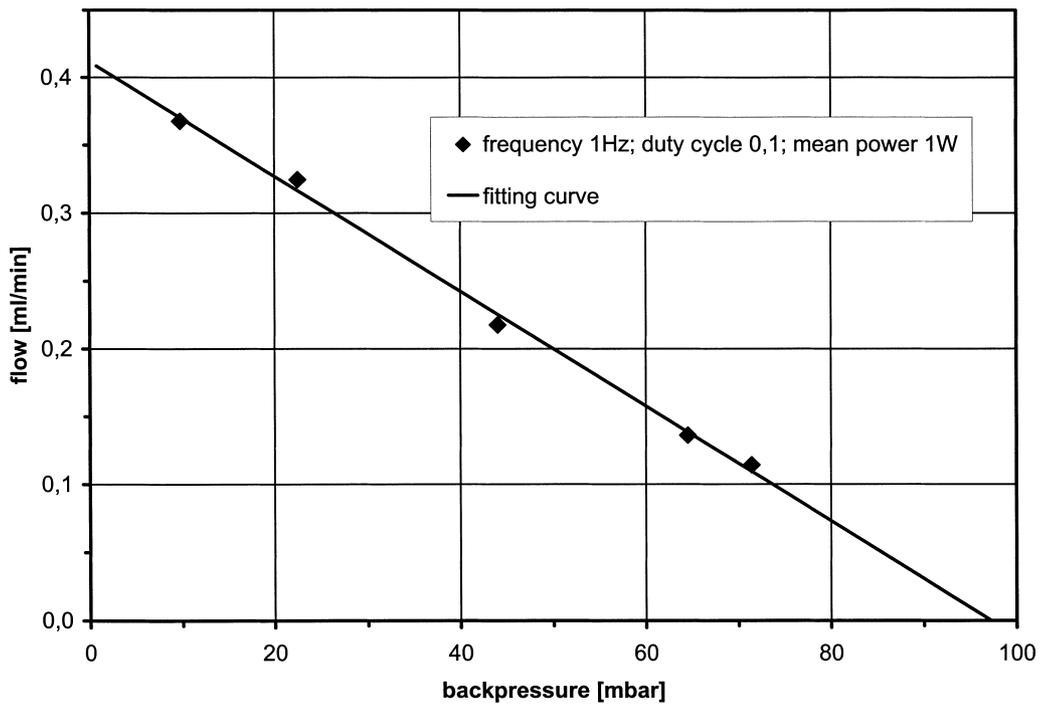
Fig. 9. Characteristic pump curve.
