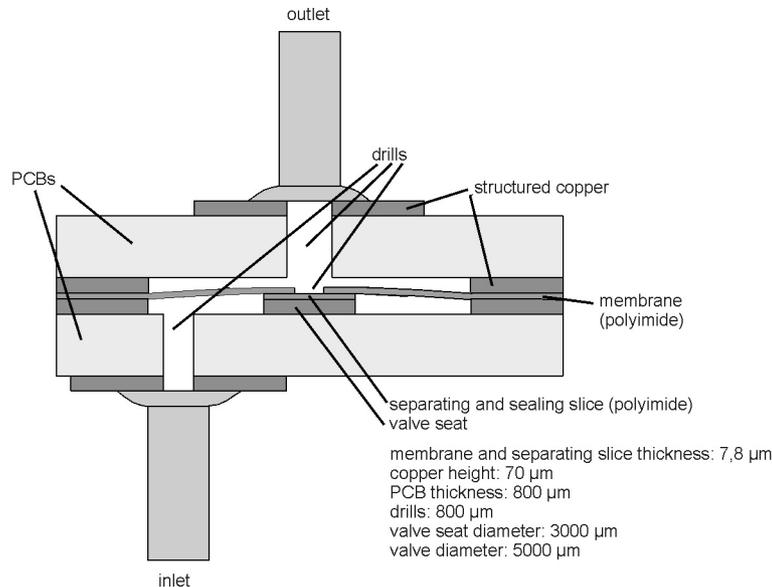
Fig. 6. Cross-sectional scheme of the passive membrane check valve.
